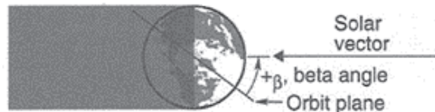
Figure 2.1. Orbit Beta Angle [14]
